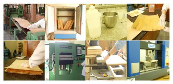
Figure 1. Stages of the manufacture and assessment of the plywood panels.
