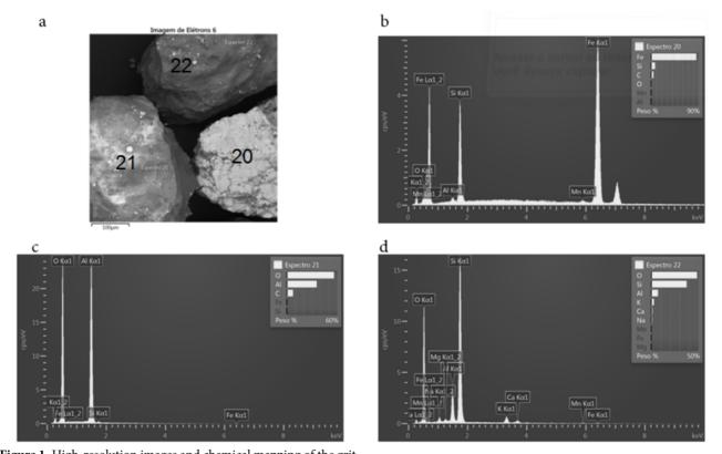
**Figure 1.** High-resolution images and chemical mapping of the grit Caption: cps/eV. Counts per second per electron-volt. Kev - kiloelectron-volt. a) spectra of the steel grit. b) EDX test results for spectrum 20 of Figure 1a. c) EDX test results for spectrum 21 of Figure 1a. d) EDX test results for spectrum 22 of Figure 1a. Spectra obtained by Tescan program.
