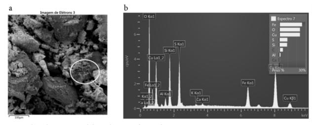
Figure 3. High-resolution images and chemical mapping of copper slag
