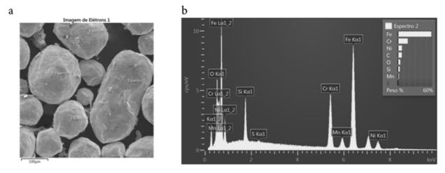
Figure 2. High-resolution images and chemical mapping of the stainless steel grit Caption: cps/eV. Counts per second per electron-volt. Kev - kiloelectron-volt. a) spectra of stainless steel grit. b) EDX test results for spectrum 2 of Figure 2a. Spectra obtained by Tescan program
