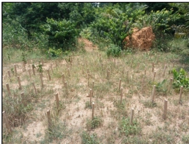
Figure 3. Positioning of thermally-modified Daniellia oliveri specimens at the decay test field.
