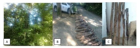
**Figure 1.** (A) Forest fragment where the experiment was conducted; (B) *sabiá* logs evaluated; (C) Logs classified (from left to right) as sound, surface attack, moderate attack, intensive attack (heavy) and failure (broken), respectively.
