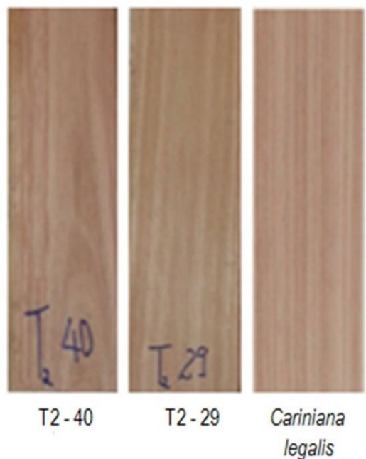
Figure 5. Visual aspect of Eucalyptus saligna wood color, treatment 2, compared with Cariniana legalis wood.
