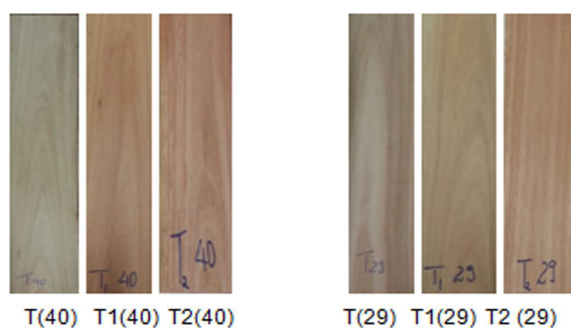
Figure 4. Visual aspect of Eucalyptus saligna wood color: control (T); treatment 1 (T1); and treatment 2 (T2).
