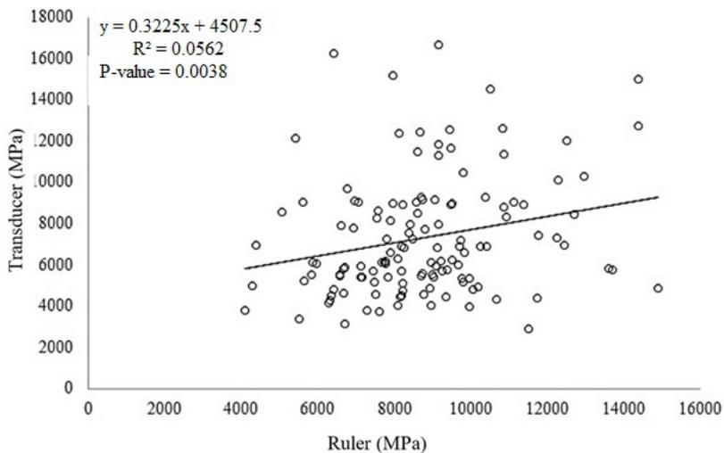
Figure 5. Correlation of transducer  $E_w$  in relation to the  $E_w$  using the fast ruler method.
