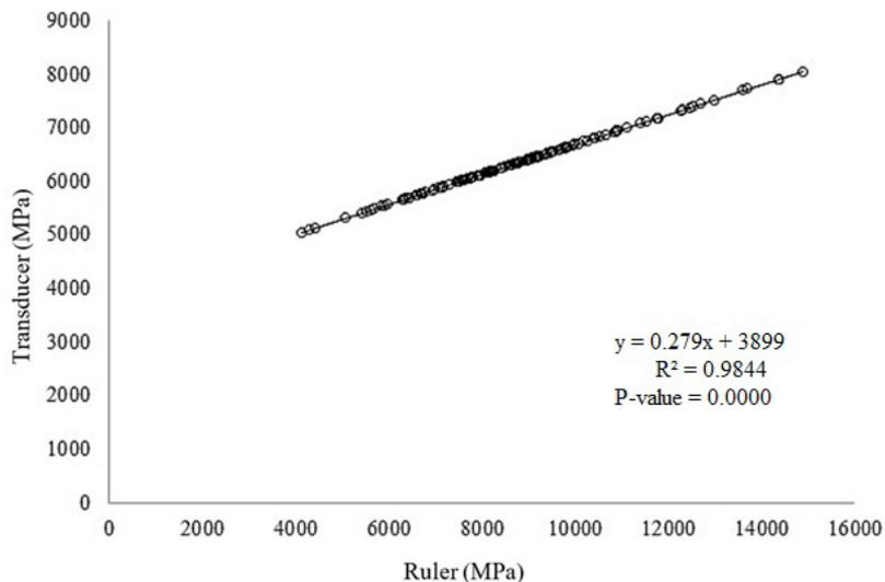
Figure 6. Correlation of transducer  $E_w$  in relation to the fast ruler  $E_w$  method.
