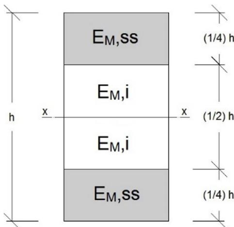
**Figure 3.** Transversal section of glulam samples with 4 laminated pieces ordered by its  $E_w$  classification.
