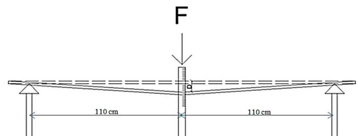
**Figure 1.** Application scheme of 30 N (F) load and displacement measure (D) to determine the stiffness of laminated wood pieces using a measuring ruler and an inductive transducer.
