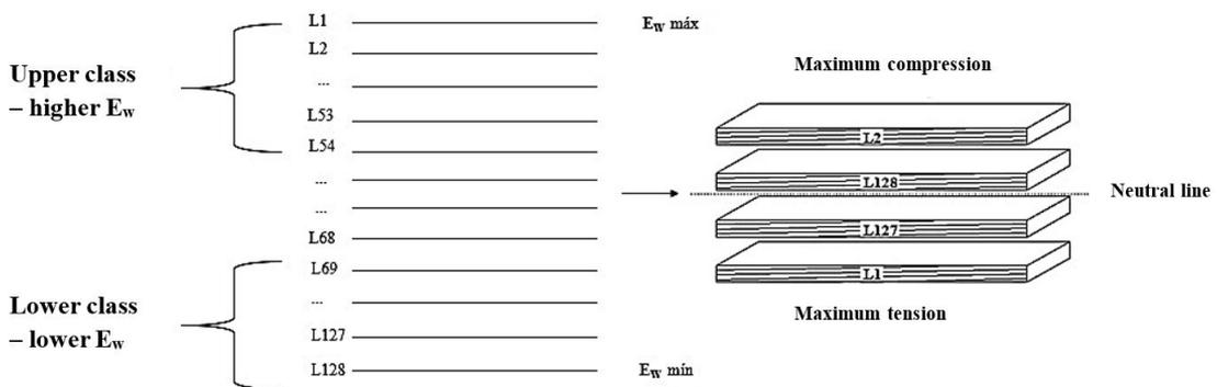
Figure 2. Distribution of laminated pieces for glulam sample composition.
