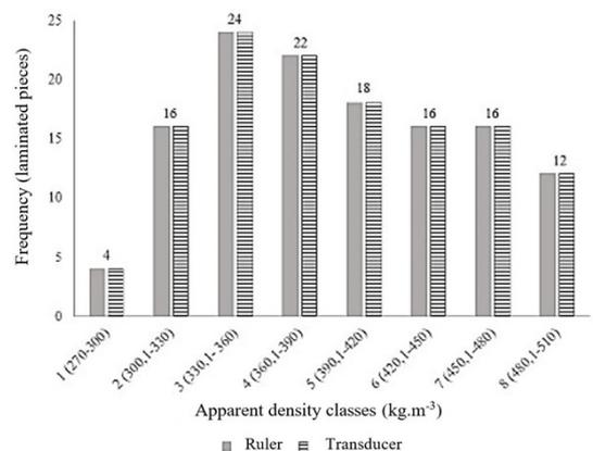
**Figure 4.** Distribution of laminated wood pieces into 8 apparent density classes.
